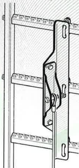
Fig. 3: Rope suspension top (Ladder)
